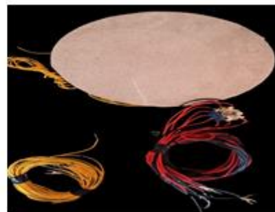
Fig.4 Heater, Ammeter, Thermo couples
