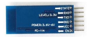
connection to other devices. The user can use it simply for a serial port replacement to establish connection
