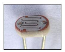
A photo resistor or Light dependent resistor is a light-controlled variable resistor. The resistance of a photo resistor decreases with increasing incident light intensity; in other words, it exhibits photoconductivity. A photo resistor can be applied in light-sensitive detector circuits, and light- and dark-activated switching circuits.
