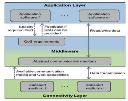
Figure 1. Plug-and-Produce Architecture
