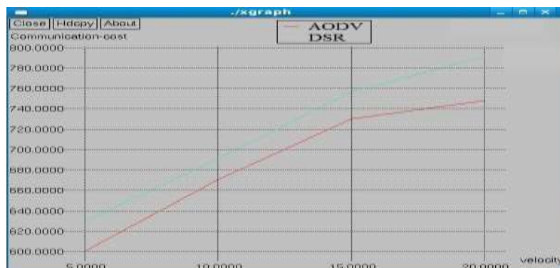
Figure.5 The Graph of the Minimization of Communication Cost Considering the Routing Protocols (AODV And DSR)
