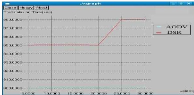
Figure.6 the Graph of Minimizing the Transmission Time Considering the Routing Protocols (AODV And DSR)
