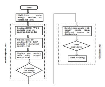
Figure: 5 Flow Chart of EWMA in Wireless Sensor
