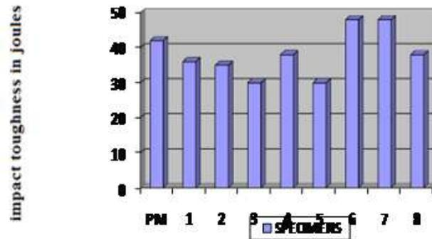
**Fig 17: Comparison of Impact Toughness of the Welds**
