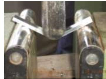
**Fig 12 (a) Bend test set up**
