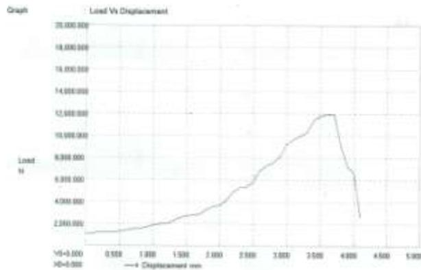
**Graph 5. Stress-Strain Diagram for Specimen 5**
