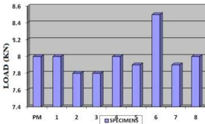
**Fig.13 (b) Comparison of Bend Load for Face Side**
