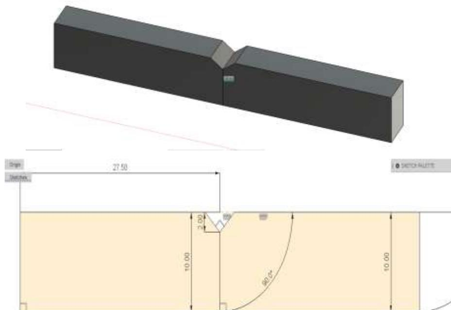
**Fig 7: Impact Toughness Test Sample**
