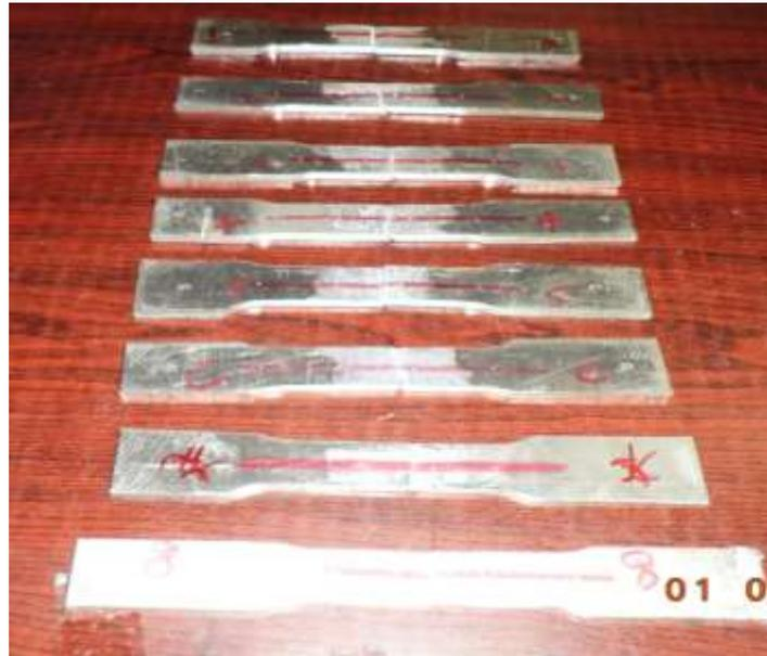
**Fig 9. Fractured Specimens after Tensile Test**
