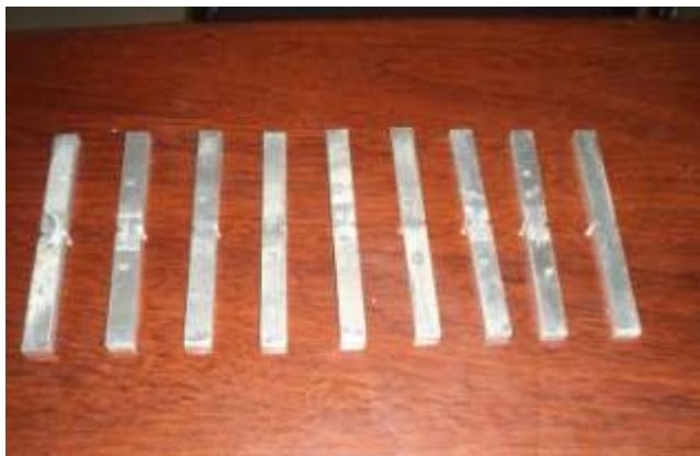
**Fig (10) a) Notch tensile test specimens**
