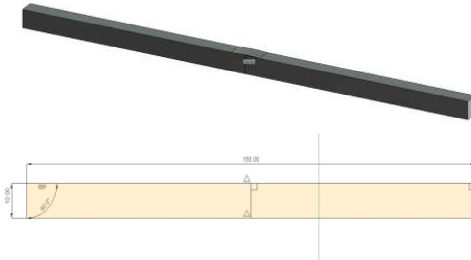
**Fig8: Bend Test Specimen**
