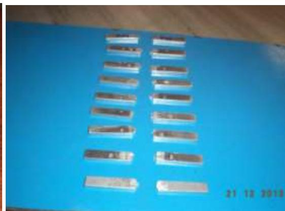
**b) Notch tensile test specimens after failure**
