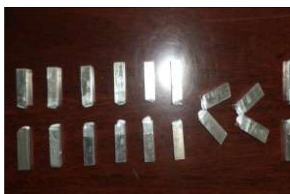
**Fig 16 a) impact test specimens      b) impact test specimens after failure**
