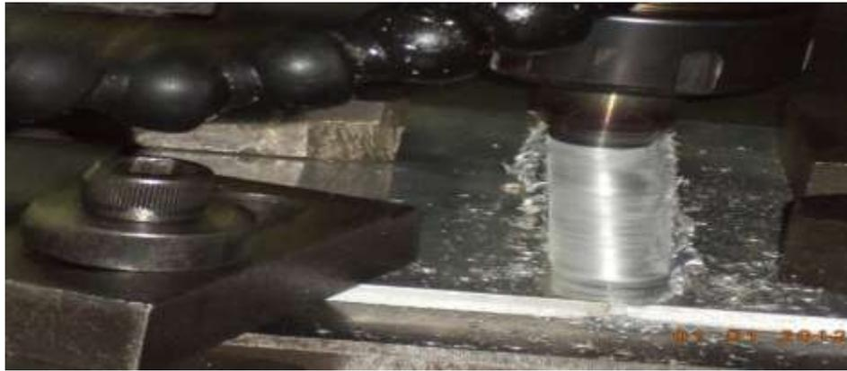
**Fig4. Experimental Set up Describing Clamping and Welding of FSW Process**
