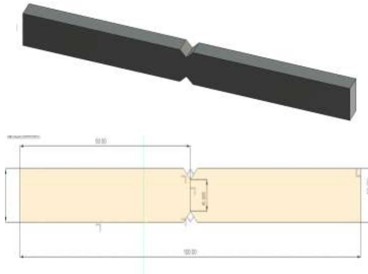
**Fig6: Notch Tensile Sample**
