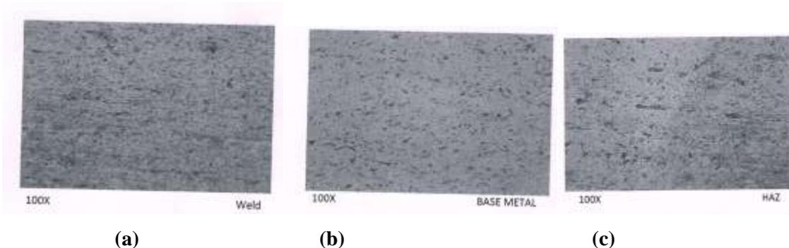
Fig 14. Various Zones Microstructures in FS Weld No.7
