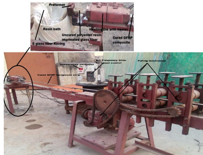
Fig.2 Indigenous Pultrusion Setup with Enlarged Heating Section
