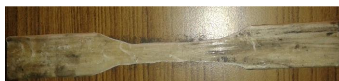
Fig. 4(a): Pultruded GFRP Composite Tensile test Specimen According to ASTM D638
