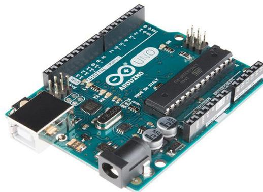
**Fig: 10. Arduino board uno R3**
