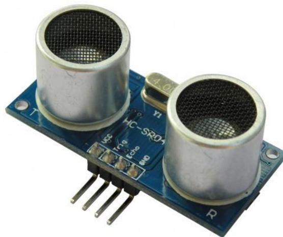
**Fig 12: Ultrasonic sensor**
